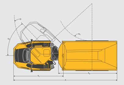
A25F: Unloaded machine with 23,5 R25 A30F: Unloaded machine with 750/65R25 \*) A25F with optional 750/65R25 tires; A30F with optional 23,5 R25 tires. \*\*) with overhung tailgate.
