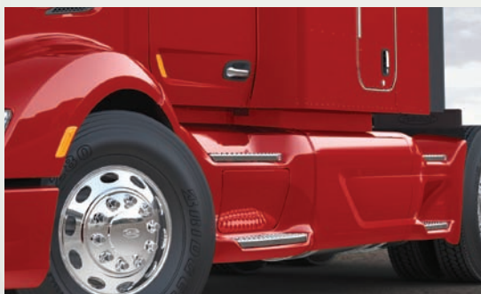
Flexible aero packages with fairings, skirts and closeouts exceed aerodynamic application requirements.
