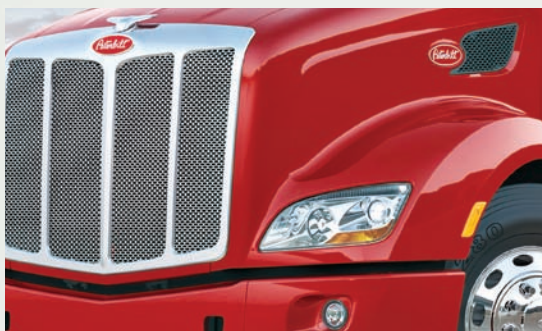
A dramatically sloped hood, bumper and air intakes streamline the overall cab shape.
