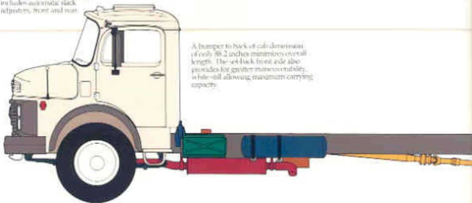
A bumper to back of cab dimension of only 88.2 inches minimizes overall length. The setback front axle also provides for greater maneuverability, while still allowing maximum carrying capacity.
