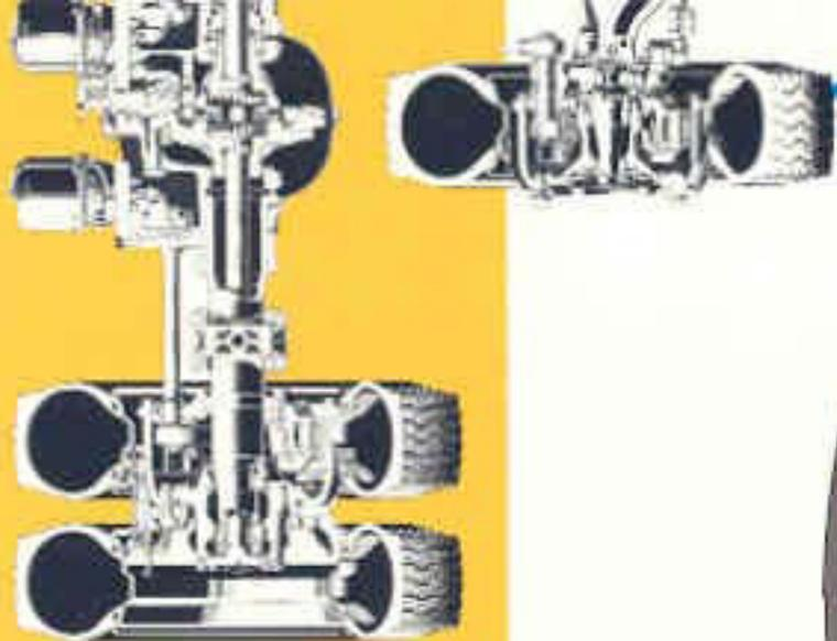
Drop legged steel alloy front axles feature large diameter, greaseable king pins for longer bushing life. Rear axles have heavy duty, box type cast metal housings with pressed in axle tubes. Ring and pinion gears are hypoid designed for smooth, efficient power to ground transmission. The standard full air brake system includes automatic slack adjusters, front and rear.
