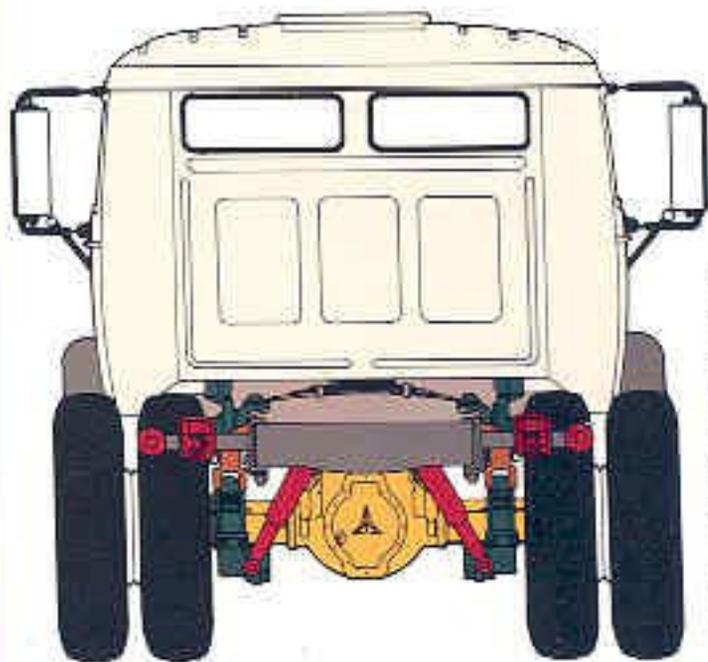
Cab suspension consists of a semi-elliptical leaf spring with two shock absorbers at the rear to reduce vibrations to a minimum — thus maintaining driver alertness and productivity. Frame mounted electrical junction boxes for simplified body wiring connections and extended frame overhangs on all wheelbases make body installation easy!
