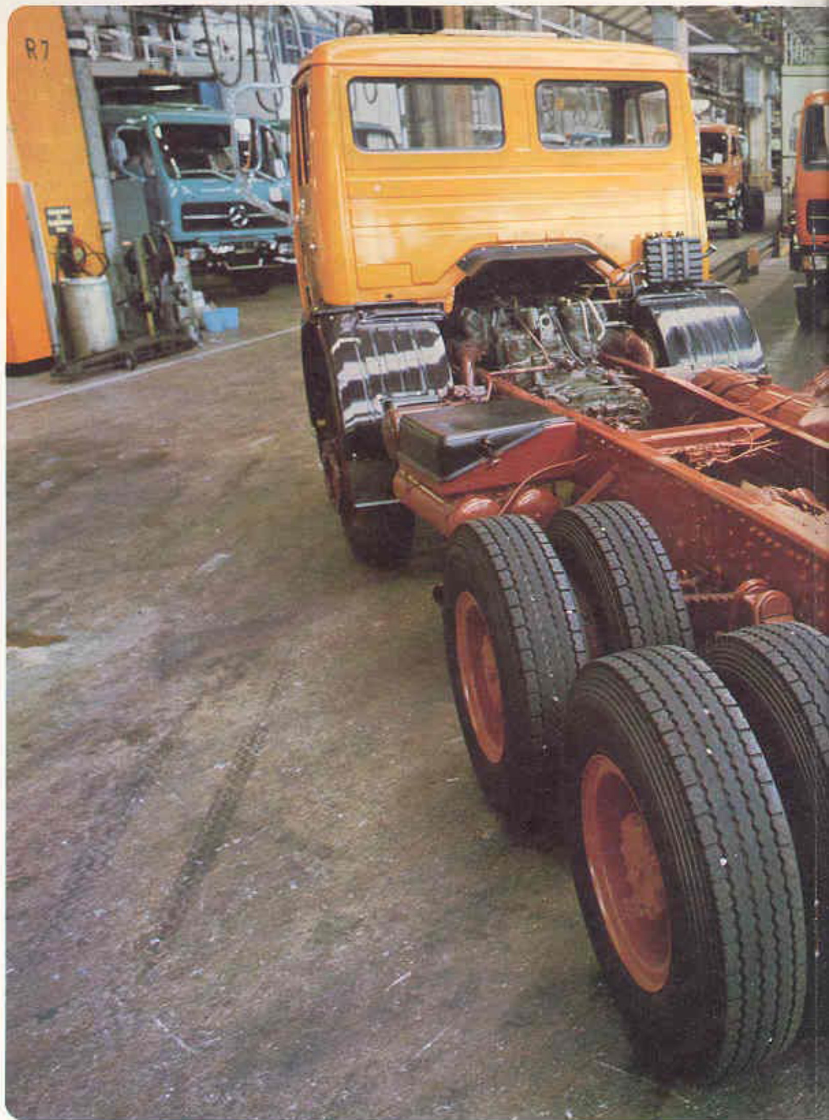
"Fish-belly" design of chassis
