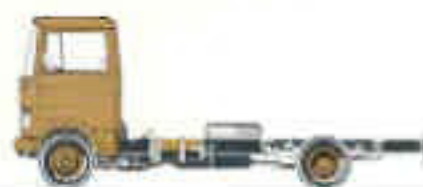
LP 913 chassis with cab Wheelbase 141.7 in. (3,600 mm) Payload and body allowance 13,100 lbs. (6,030 kg)
