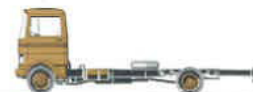
LP 913 chassis with cab Wheelbase 165.3 (4,200 mm) Payload and body allowance 12,910 lbs. (6,855 kg)
