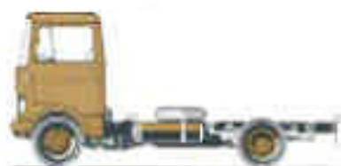
LP 913 chassis with cab Wheelbase 126 in. (3,200 mm) Payload and body allowance 13,500 lbs. (6,130 kg)
