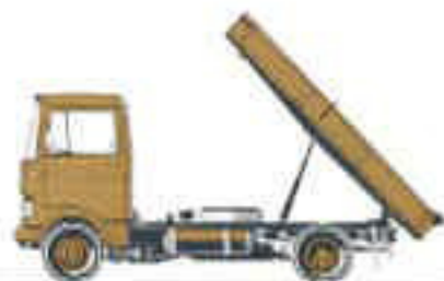
LPK 913, topper Wheelbase 126 in. (3,200 mm) Recommended body size 137.8 x 82.7 x 11.8 in. (3,500 x 2,140 x 400 mm) Payload 11,000 lbs. (5,015 kg)
