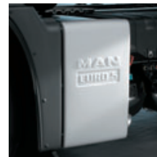
Silencer with SCR catalyst for Euro 5.
