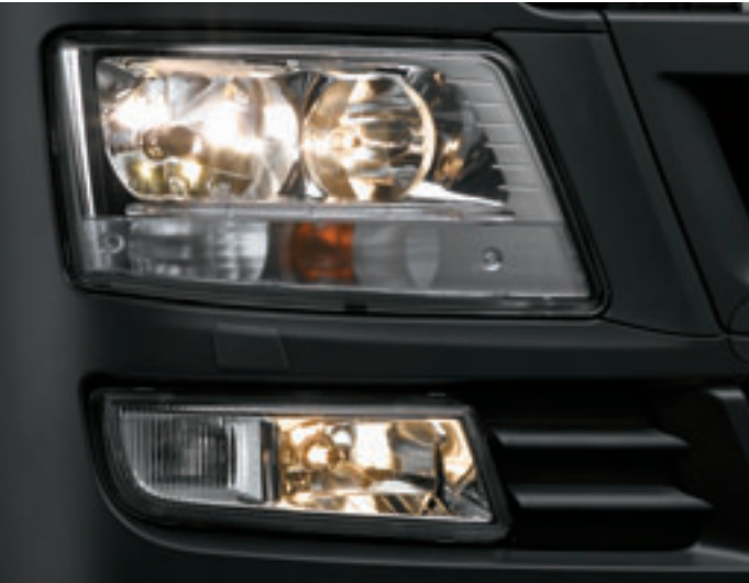
Headlights with free-form reflectors, Xenon dipped headlight.
