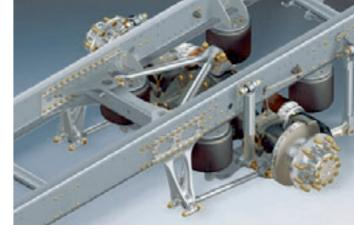
4-bellows rear-axle air suspension for the TGM. Optional heavy-duty rear axle, load capacity 11.5 tonnes.
