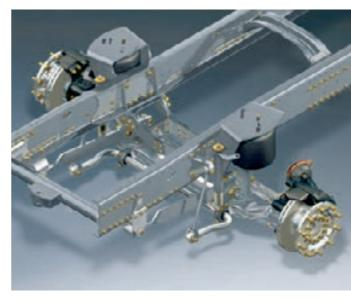
Front-axle air suspension for the TGM.
