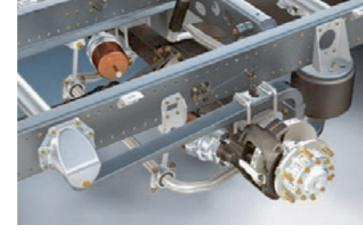
2-bellows rear-axle air suspension for the TGL
