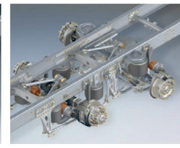
Steered trailing axle with air suspension for the TGM.
