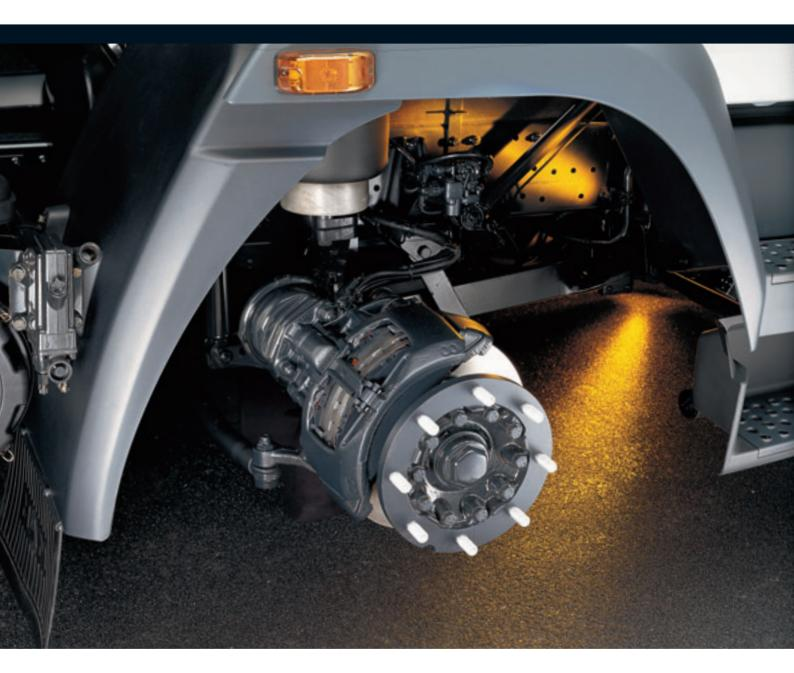
**RIDE SAFELY, BRAKE SAFELY.** When it comes to braking distance, the M2000 Evolution's motto is "a little is more." That's why it has air-actuated and internally ventilated disk brakes on the front axles. Low-abrasive s-cam and/or wedge drum brakes with automatic brake shoe readjustment make for reliable performance at the rear. On all-wheel drive versions, drum brakes are used on every axle.
