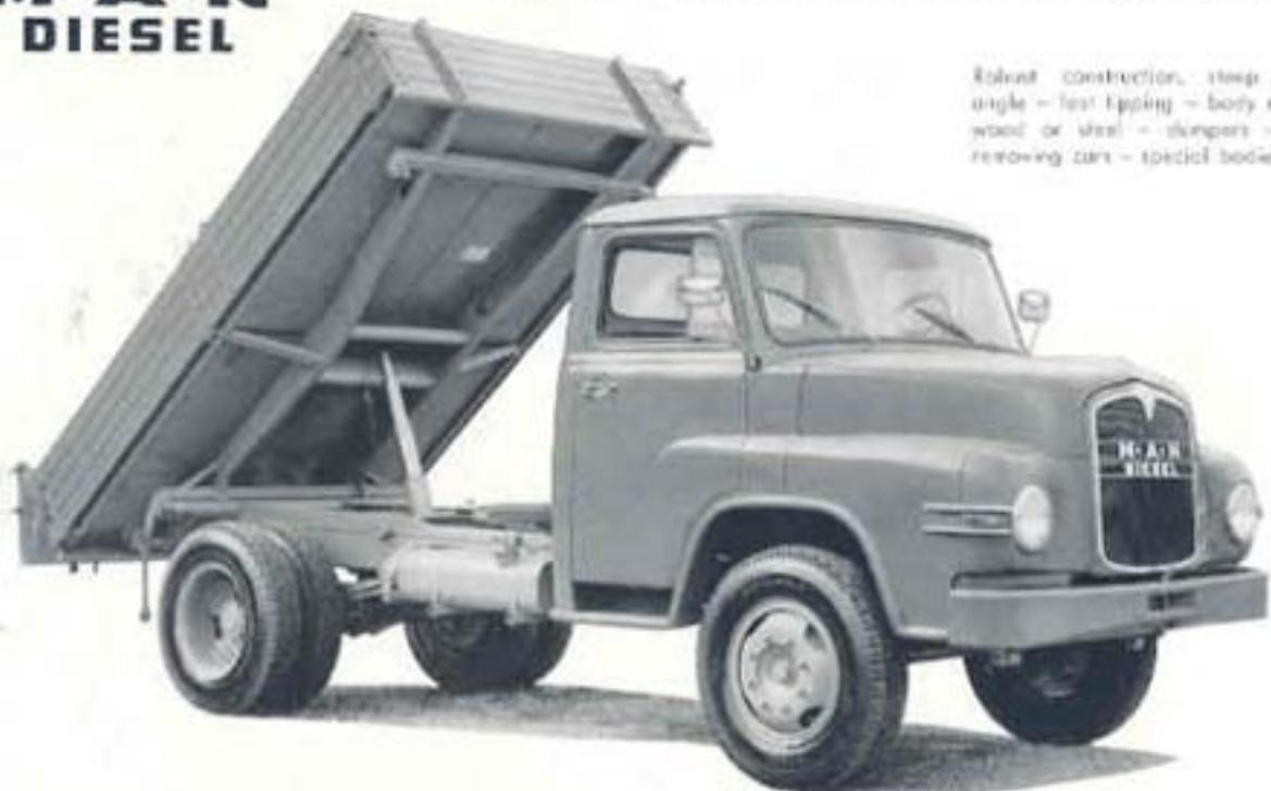
Robust construction, steep tipping angle - fast tipping - body made of wood or steel - dampers - safety running gear - optional bodies.
