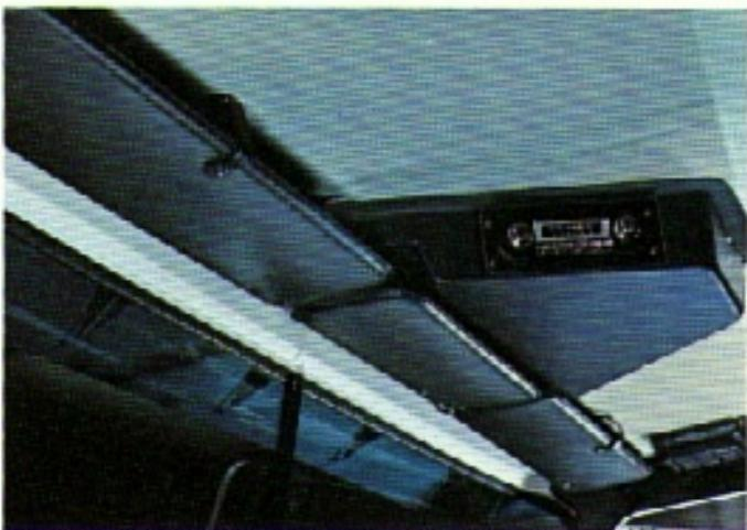
The headliner provides overhead and roof-mounted antenna locations. Various audio systems are available to specification. An effective sound deadener, the headliner is a two-piece type for easy removal if required.
