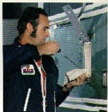
Oil fill and dip stick located for easy servicing from side of cab.
