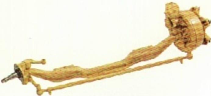
Mack's FAW537 front axle is a 12,000-pound (5,443 kg) capacity Reverse-Elliott, drop-forged, I-beam construction for both toughness and lightweight. Mack's selective steering geometry permits sharper turns with less effort.
