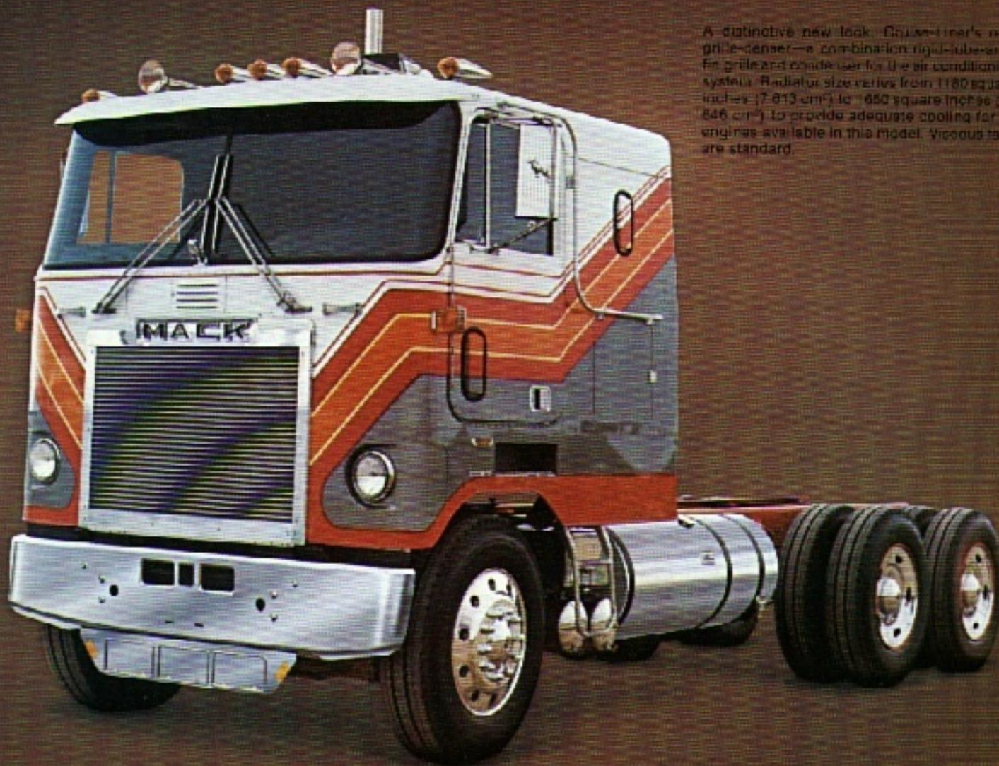
A distinctive new look. Mack's new grille-denser—a combination liquid-cooler and fin grille and condenser for the air conditioning system. Radiator sizes range from 1180 square inches (7,813 cm<sup>2</sup>) to 1,650 square inches (10,846 cm<sup>2</sup>) to provide adequate cooling for all engines available in this model. Viscous fans are standard.
