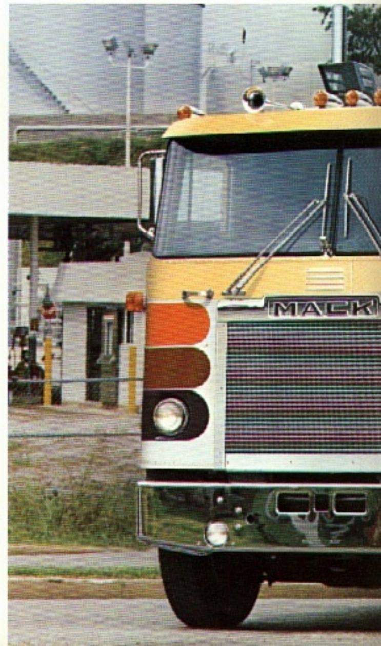
Double-arm pantograph wipers provide a wipe area of 1500 square inches (9,678 cm<sup>2</sup>) with washer outlets mounted directly on the wiper arms. Note optional exterior visor for extra protection from the sun.
