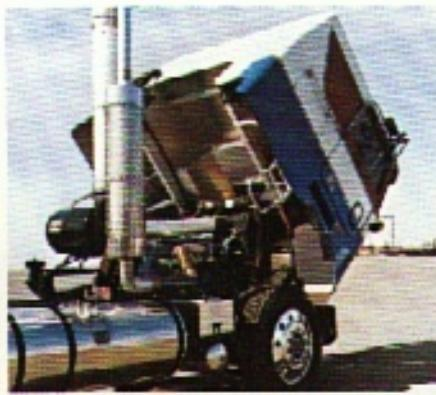
To make maintenance as simple as possible, cab has a maximum hydraulic tilt for easy access to engine and other components. Underside of cab is clean and uncluttered; there is no exposed insulation to get oil-soaked or soiled.
