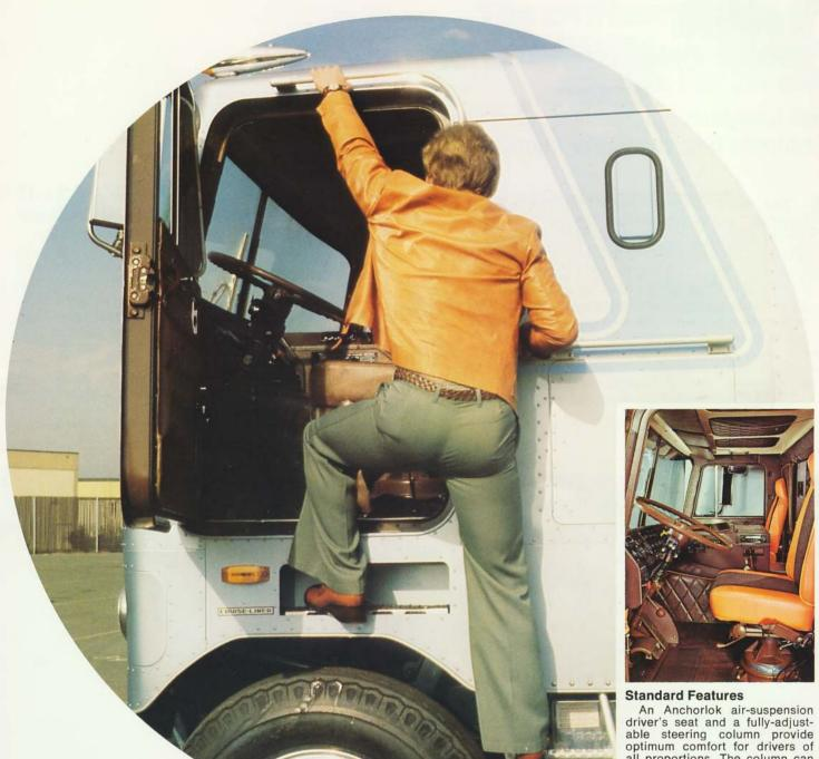
An Anchorlok air-suspension driver's seat and a fully-adjustable steering column provide optimum comfort for drivers of all proportions. The column can be moved up & down and also tilted to suit any driver preference; and is secured by a camtype locking lever at the lower edge of the dash.
