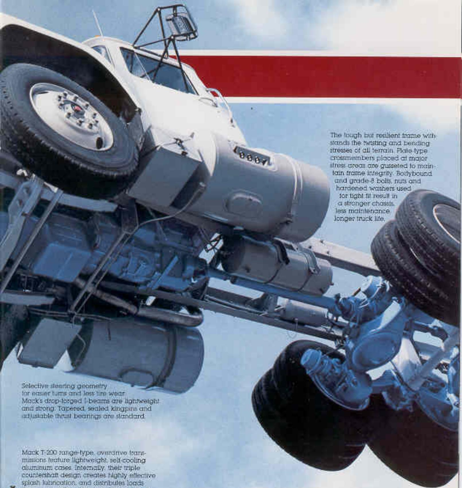
The tough but resilient frame withstands the twisting and bending stresses of all terrain. Flare-type crossmembers placed at major stress areas are gusseted to maintain frame integrity. Bodybound and grade-8 bolts, nuts and hardened washers used for tight fit result in a stronger chassis, less maintenance, longer truck life.
