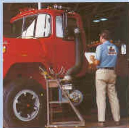
Pressure testing guarantees cab sealing against heat, cold, moisture and noise. Additional floor undercoating helps to further reduce cab interior sound levels.
