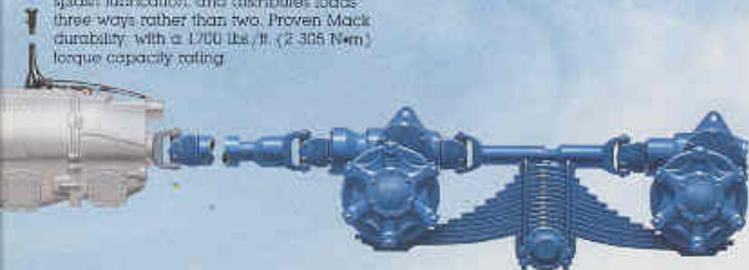
Mack bogies for highway use handle from 34,000 pounds (15,422 kg) to 44,000 pounds (19,958 kg). Parallelogram design allows maximum articulation, and the unique Mack inter-axle power divider automatically delivers increased torque to the axle having the greatest traction. Vendor suspensions are also available.
