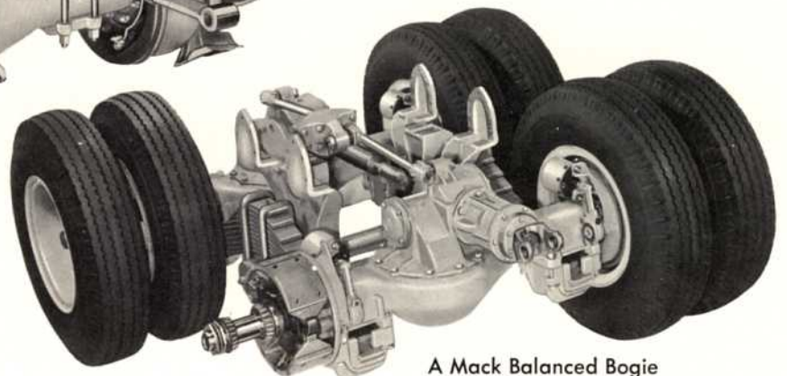
Mack rear axles available in hypoid and Dual Reduction drive
