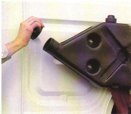
Radiator expansion tank is externally located for easy access—with cap positioned for effortless checks and fill-ups.
