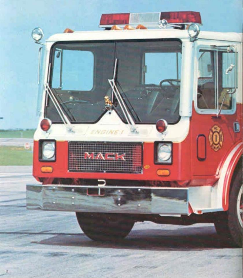
The MC Fire Pumper from Mack, the company that has earned the firefighter's confidence. Clean lines, excellent visibility, and great maneuverability highlight this first-run, attack-type custom pumper. Extensive use of galvanized steet, fiberglass and aluminum makes the MC Fire Pumper one of the most rust-resistant vehicles ever offered to the fire services. Fire-engineered to your demands, because people rely on you. Mack-engineered to our demands, because you rely on us.
