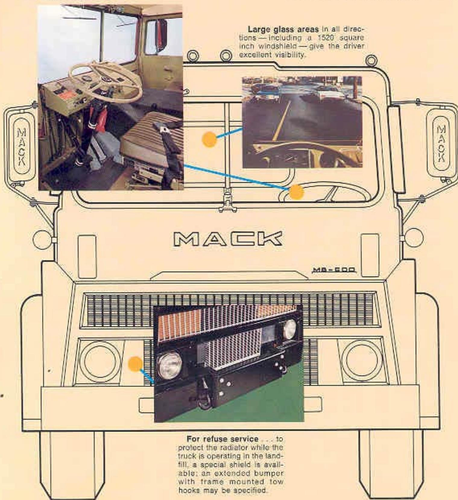
For refuse service . . . to protect the radiator while the truck is operating in the landfill, a special shield is available; an extended bumper with frame mounted tow hooks may be specified.
