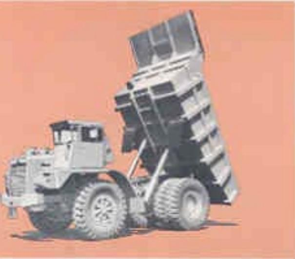
Spacious single man cab showing driver access, 3-way adjustable seat, human engineered controls and instruments, wide view visibility taking full advantage of cab forward position.
