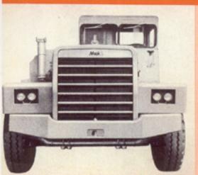
Adequate cooling under the most rugged and adverse operating conditions is effected by giant continuous-finned flat-tube type radiators with frontal areas up to 2330 square inches.
