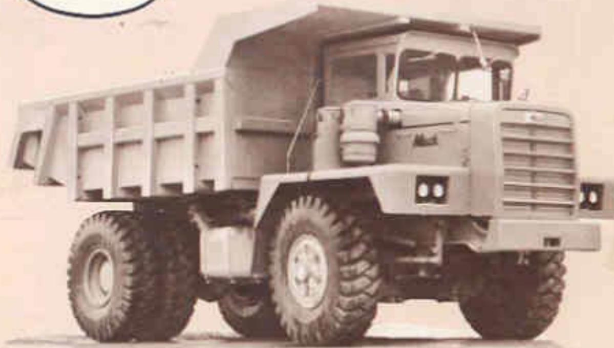
MACK MODEL M-35X is a four-wheel, diesel powered, end-dump truck with an increased payload capacity due to a saving in vehicle weight.
