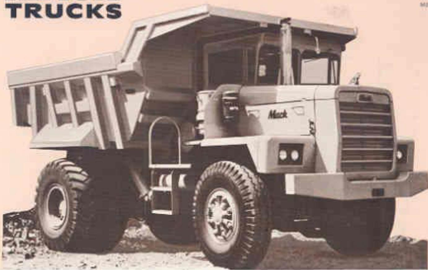
Dependability and low cost operation in the medium-capacity Off-Highway dump truck field is reliably met by the Mack Model M-25X with an All Mack power train. Standard engine is the Mack EMDT 673C, a turbocharged six cylinder diesel which develops 250 horsepower. This engine has the same sound thermodynamic diesel features that have made Mack engines world famous for reliability, low maintenance and economical service.
