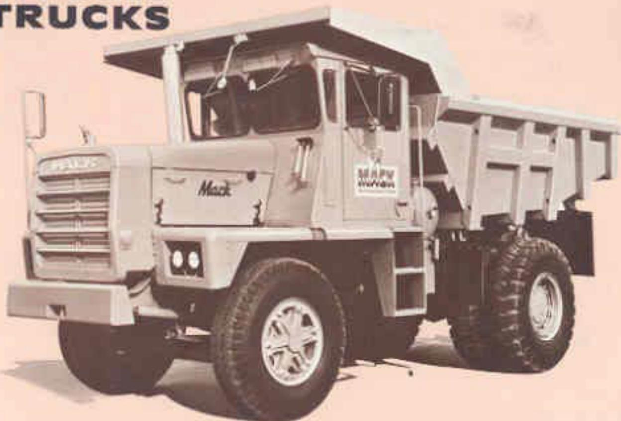
Dependable hauling in the 20 ton off-highway dump field at minimum operating cost is offered by Mack model M-20X. This diesel-powered four-wheel truck is designed specifically for use in the contracting, mining, and quarrying fields. Increased payload capacity is obtained by engineering improvements and reduction in vehicle weight.
