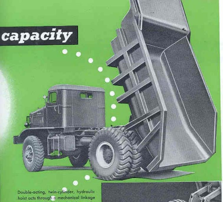
Double-acting, twin-cylinder, hydraulic hoist acts through a mechanical linkage to provide a 70-degree dumping angle. Diameter of the cylinders is 10 inches, stroke is 24 inches. Raising or lowering speed of the hoist is 15 seconds.
