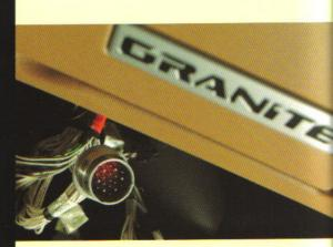
Attaching body to truck is now easier than ever with our Body Link connectors. Conveniently located under the hood and dash panel, Body Link eliminates wire cutting and splicing. Just plug in and go.
