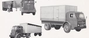
Built in sizes from 20,000 lbs. to 28,000 lbs. G. V. W. as straight trucks, and as a tractor in the 40,000—53,000 lbs. G. C. W. range.
