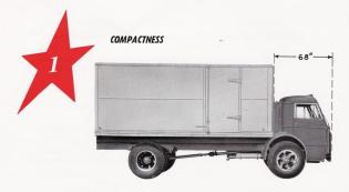
COMPACTNESS — 12 inches shorter overall length than other cab-over-engine designs and up to 50 inches shorter than conventional types — that's proof that the Mack Cab-Forward D-series models are the most compact. Having a dimension of only 68 inches from front bumper to the back of the spacious 75-inch-wide three-man cab, Mack D models, for any given size body or tractor-trailer combinations, will be a good 12 inches shorter in overall length and other C.O.E.'s, will permit a foot longer body.
