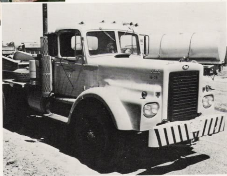
AFTER INSTALLATION OF CLARIBEN HOOD
