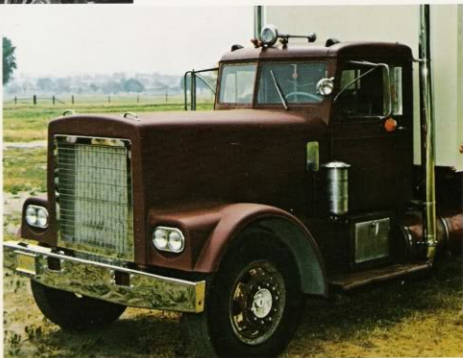
AFTER INSTALLATION OF CLARIBEN HOOD
