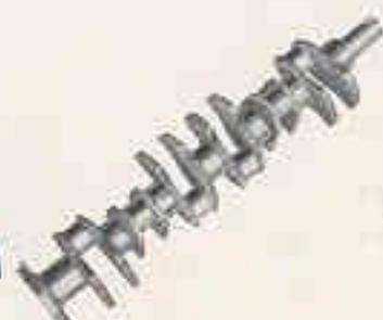
For smooth even running, longer bearing life, the large, seven-bearing crankshaft, electrically case-hardened, is fully counterbalanced by 12 integrally forged counterweights.
