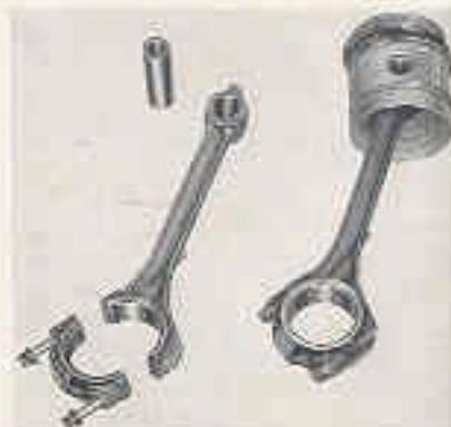
Easily removable connecting rods are of angle split type; provide greater strength and stiffness than conventional types.
