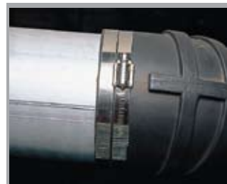
Double clamping provides extra engine protection.
