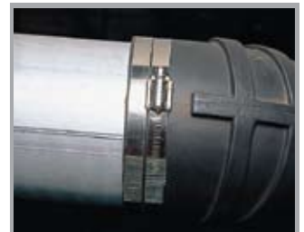
Double clamping provides extra engine protection.
