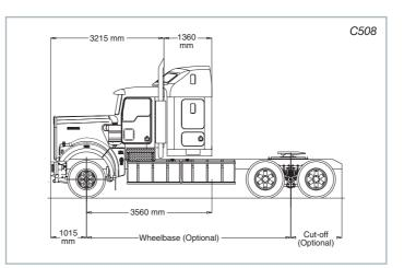
The C508 features a robust chassis, with a traditional hood configuration to suit on or off-highway heavy haul applications.
