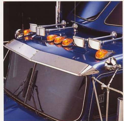
Round or rectangular horns and marker lights. Painted fiberglass or stainless steel sunvisor. Factory-installed antenna and hookup for cellular phone.
