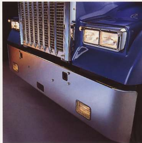
Traditional Kenworth gullwing or rectangular Texas-style chromed steel bumper. Stainless steel eyebrow over headlights. Screen for fog lights.
