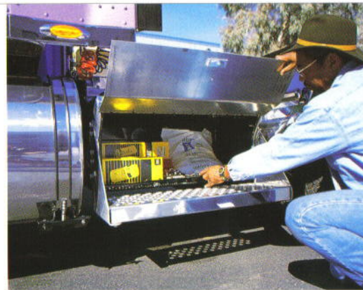
Optional Kenworth-built aluminum or steel diamond-plate toolboxes can be located under the cab or in back of the fuel tanks.
