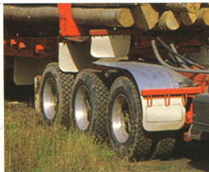
Kenworth is one of the few manufacturers to build effective tri-drives – offering the pulling power of a 6 x 6 for less money and without the hassle of a transfer case or the raised front end of a front drive axle.
