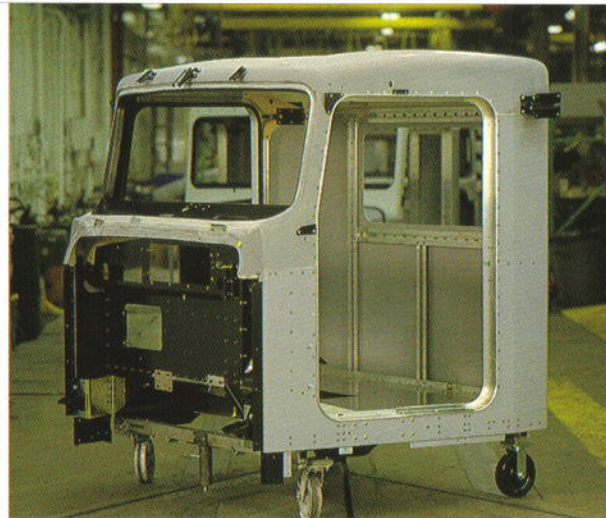
Coil-coated aluminum panels and a one-piece fiberglass roof, supported by an aircraft-grade aluminum alloy frame, produce a lightweight yet durable cab that is virtually immune to rust.
