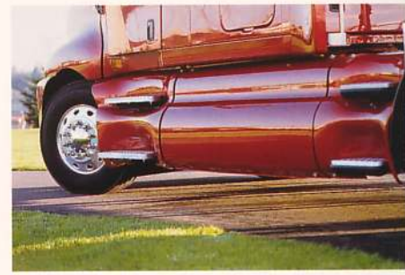
Standard under-cab fairings reduce turbulence and splash/spray, advancing the art of aerodynamics as well as public safety.
