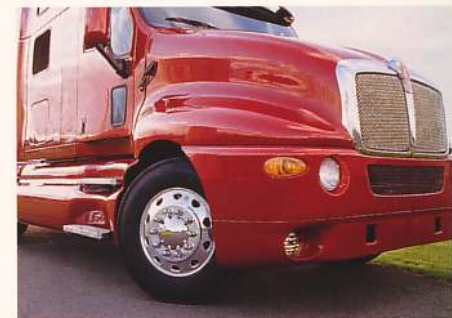
The T2000 features separate upper and lower bumper assemblies, reducing service and replacement costs.
