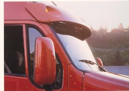
An optimally curved windshield, sloped precisely 30 degrees, directs wind upward and over the vehicle in a fluid, uninterrupted stream. Even the exterior mirror housings are shaped to slice smoothly through the air.
