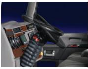
Tilt and telescoping steering column.
