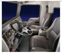
The fully-trimmed standard Pinnacle interior is shown with the optional Kenworth Air Cushion Plus high back driver seat and Kenworth Toolbox Plus passenger seat. Also shown is the workstation between the seats for added convenience
