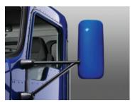
Heated and electronically-adjusted aerodynamic mirrors.
