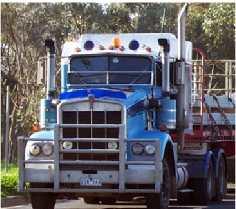
KW SAR with large radiator for large HP engines with wide radiator grille
