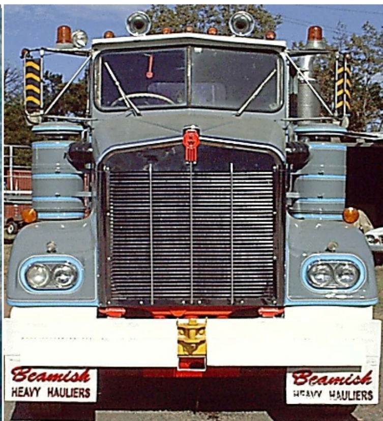
KW SAR with large radiator for large HP engines with wide radiator grille
