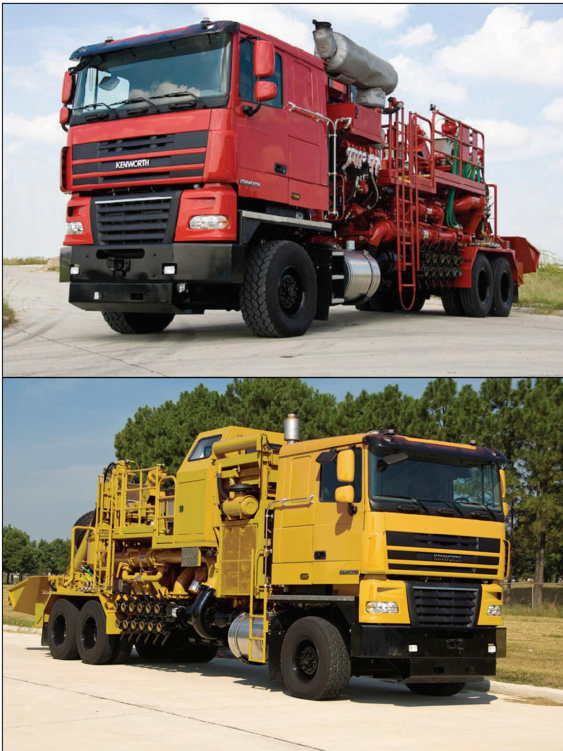
The K500 is a combination of the C500 drivetrain with a modern, PACCAR COE cab. This configuration addresses the need for an on/off-highway vehicle with improved visibility and more cab space than provided by conventional models. The resulting unit is a shorter, more maneuverable truck or tractor with the mobile off-highway characteristics that make this Kenworth highly desirable, whatever the application.
