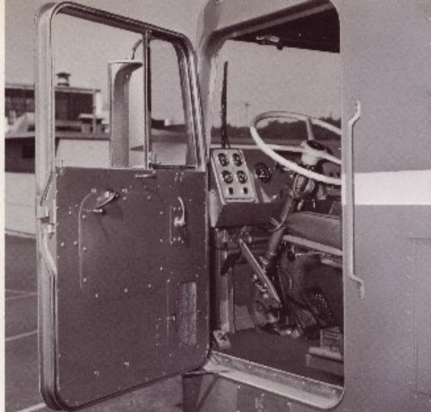
Bulkhead door features continuous weather stripping and extruded aluminum frame, piano-type hinges.
