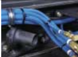
Kenworth offers wirebraided hose for its air brake systems – an extra that pays off in peace of mind when your application takes you miles from anywhere.
