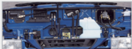
Lockable front panel Facilitates repairs and maintenance without tilting cab
