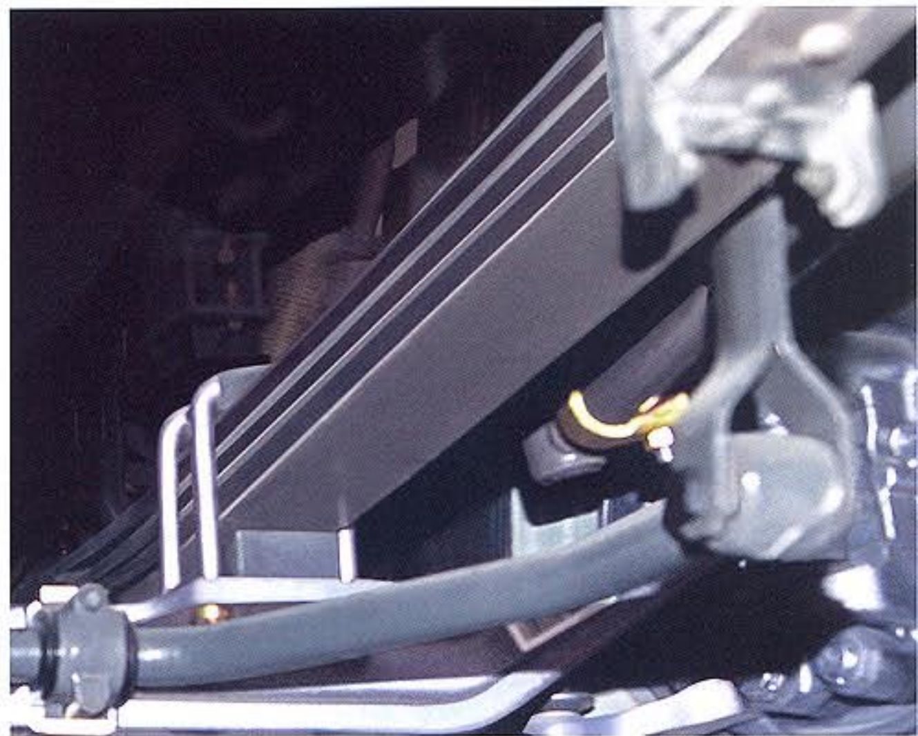
少片簧。片与片之间的减摩片能有效降低噪声。 Saving leaf springs, the friction-reducing plates between springs can reduce noise effectively.
