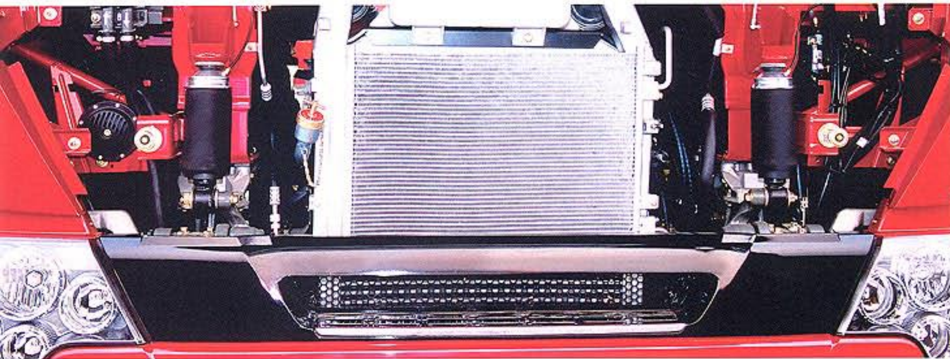
驾驶室悬置采用四点空气弹簧全浮式结构，翻转轴为模锻整体成型，四轴承连接，转动灵活，使用可靠。 The cab suspension features a four-point full-floating air suspension structure. The tilting shaft is integrally forged, with four bearings connected with each other, making it very flexible and reliable.
