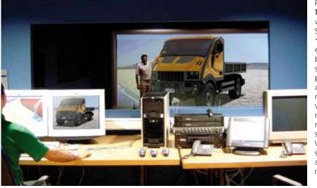
From the first sketches, T-REX has been fully designed with computer. Steeve says: "Thanks to the virtual engineering systems, we have been able to keep an eye, since the beginning of the project, on all the different aspects of the vehicle and maintain its characteristics: visibility and ergonomics tests, mechanical equipment, maintenance, and of course, structure resistance. We have realized a particular study to improve the aerodynamic flow and to reduce consumption".
