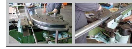
The roll-bar is shaped in 3 dimensions thanks to a specific tube benders use.
