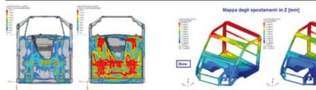
At the right, a conventional floor. On the left, reinforced steel floor, capable to withstand to 5 +1 G!
