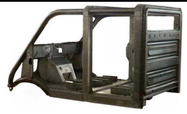
The new BREMACH vehicle is made with a cell of adaptive modular space frame
