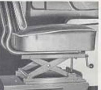
Back seats are provided in some heavier-duty models, and are easily removable and adjustable for height, as well as for length, if required.
