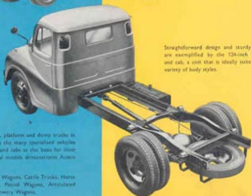
The 115-inch wheelbase chassis can be provided with damping gear, or employed as the motive unit for many types of articulated vehicles of which this pantechnicon is a good example.
