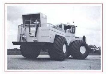
The Model 'N' can be used as a drill carrier as shown above or as a fuel tender as on the left. Other uses in various industries such as a cable carrier for mining applications demonstrate ARDCO's ability to adapt the Model 'N' to your requirements.
