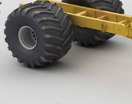
You won't find any modified truck axles on a TerraGator. Rugged Axle Tech™ off-road axles, designed specifically for use with high-flotation tires, carry even the heaviest load with strength and stability. In fact, they handle the highest load ratings in the industry. And the dynamic, load-sensing steering features an anti-kickback design that keeps the shock loads of rough ground from transferring from the axles to the steering wheel and the operator.
