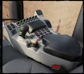
Operations are made even easier with a joystick that can be used to manage ground speed and serves as a convenient location for the master apply switch to control application functions.
