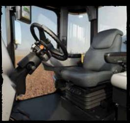
Our semi-active deluxe seat is now standard on all TerraGators for improved operator comfort. The seat allows for real-time automatic dampening force to match field terrain and operator preference.
