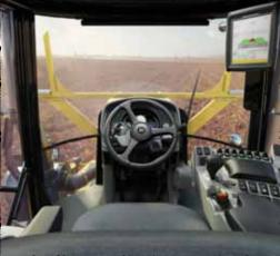
The boom control switches and additional presets are laid out so they are within easy reach of the operator, with the most commonly used switches logically placed.
