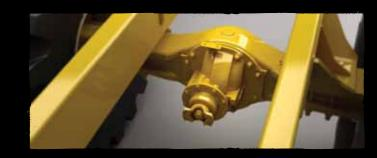
TerraGator's industry-leading paint and finish process provides years of protection from rust and corrosion. The chassis is shot blasted, degreased and phosphate treated prior to painting for maximum paint adhesion and corrosion resistance.
