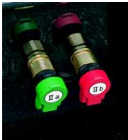
Clearly marked hydraulic connections.
