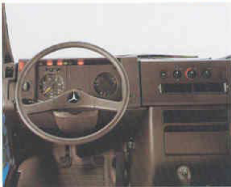
Clearly arranged instruments with optimum, non-reflecting night illumination with back-light design.
