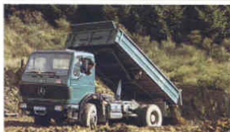
Dumpers work reliably in bad terrain, too, if they have all-wheel drive. Maneuvrability is maintained at all times due to the transmission of power to all four wheels, and the differential lock which can be engaged at will.
