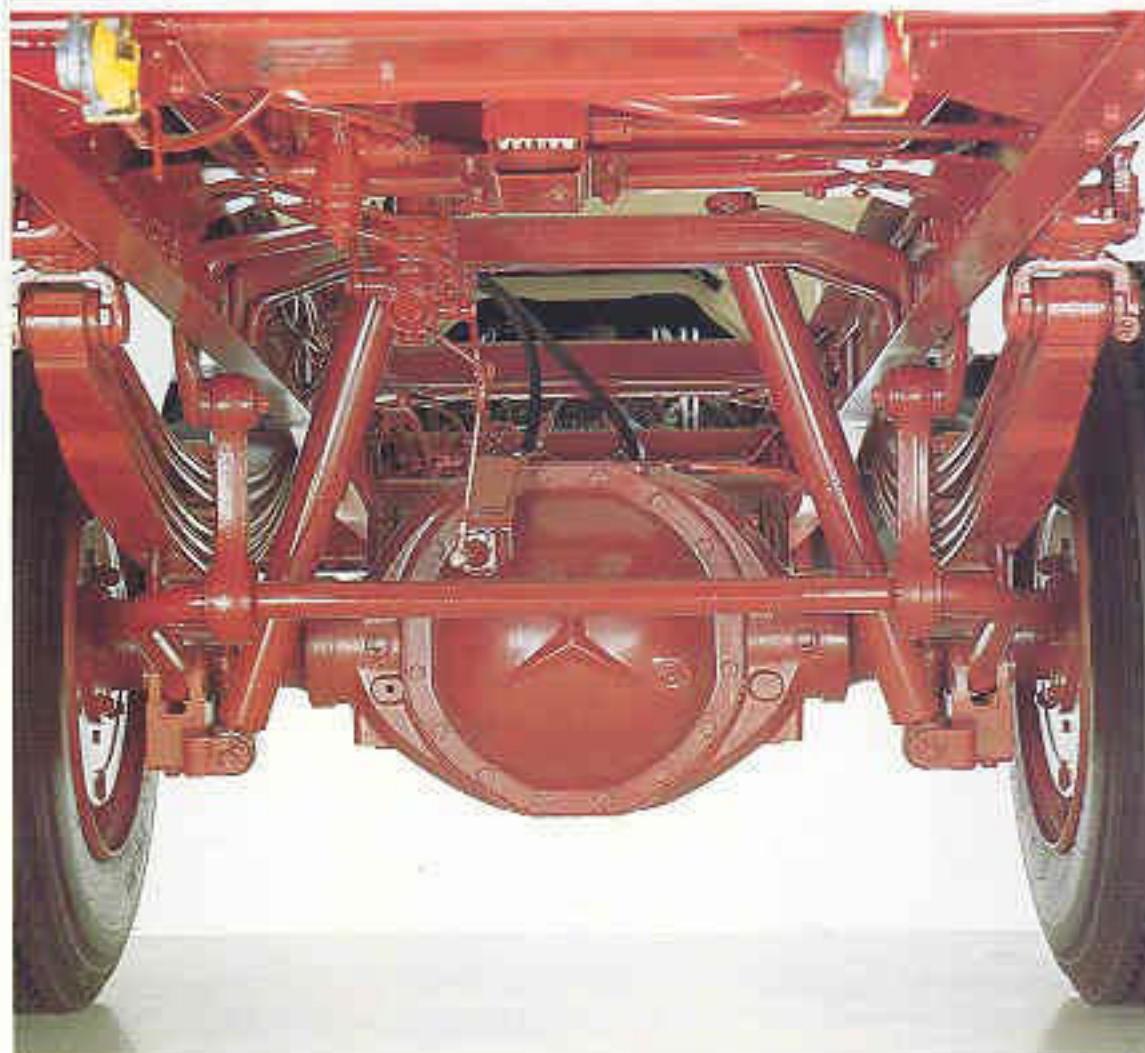
Top: All-wheel drive front axle with hypoid gearing. High load-bearing capacity, minimum dead weight.
