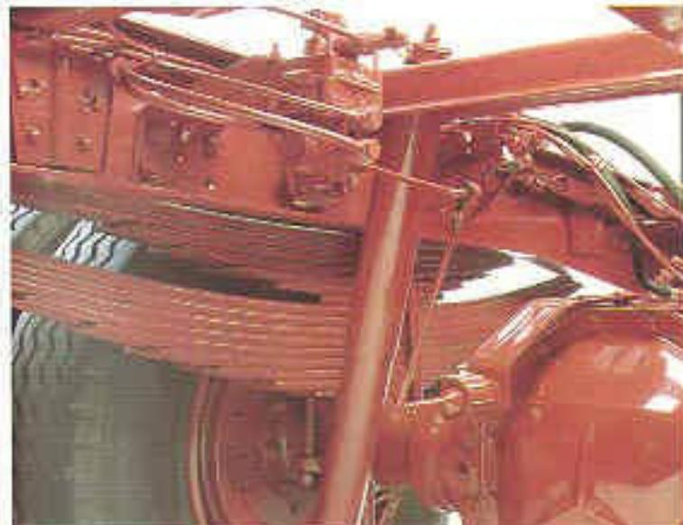
Vehicles from 121 GVW upwards are fitted with Mercedes-Benz power steering. Safe and accurate steering is guaranteed at all speeds since the driver can feel changes in the condition of the road surface and in tyre adhesion directly from the wheel. The power steering is particularly helpful for driving slowly or for manoeuvring, since even gentle turning pressure on the steering wheel causes the steering nut to activate the control valve.
