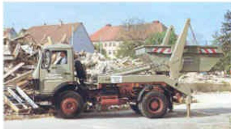
Medium-heavy two-axle chassis can be fitted with all kinds of special bodies, such as here for the picking up and transport of demolition troughs.
