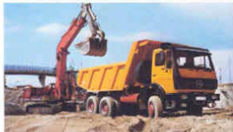
Mercedes-Benz chassis are suitable for any kind of body. Reputable body manufacturers fit the chassis with, for instance, tipping troughs for transporting gravel, sand, etc.
