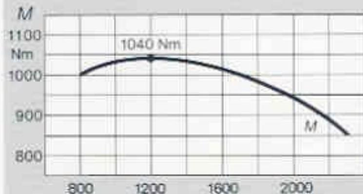
The curve clearly shows that maximum torque is available at low engine speeds. Moving off from a stationary position is made easier, and even steep inclines can be mastered with the engine speeds in the low-consumption range.
