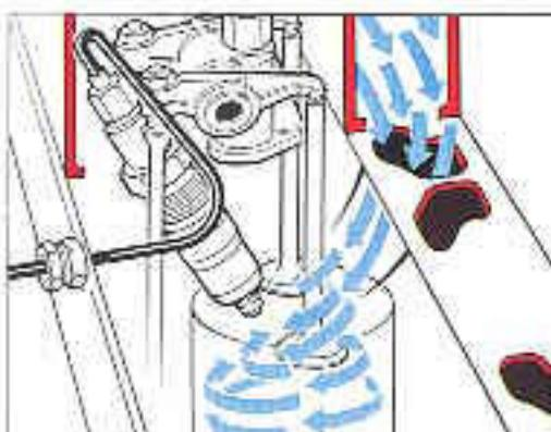
Operating method of the Mercedes-Benz direct-injection system
